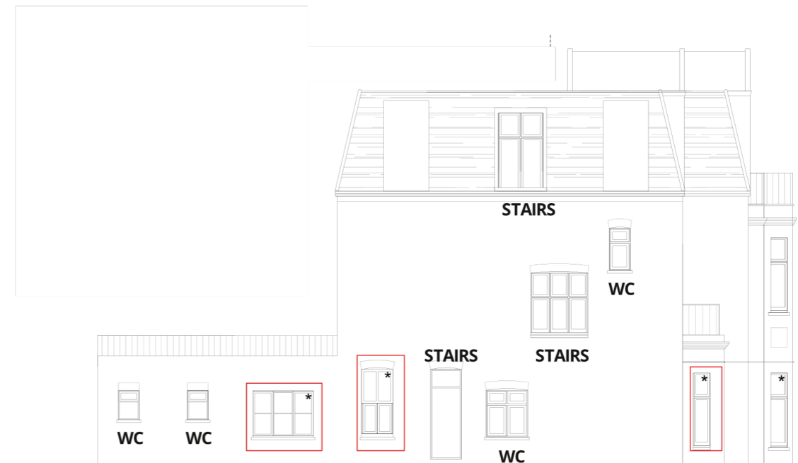
GROUND FLOOR PLAN AND WESTERN FACADE OF 192 GOLDHURST TERRACE ILLUSTRATING THE HABITABLE WINDOWS.
